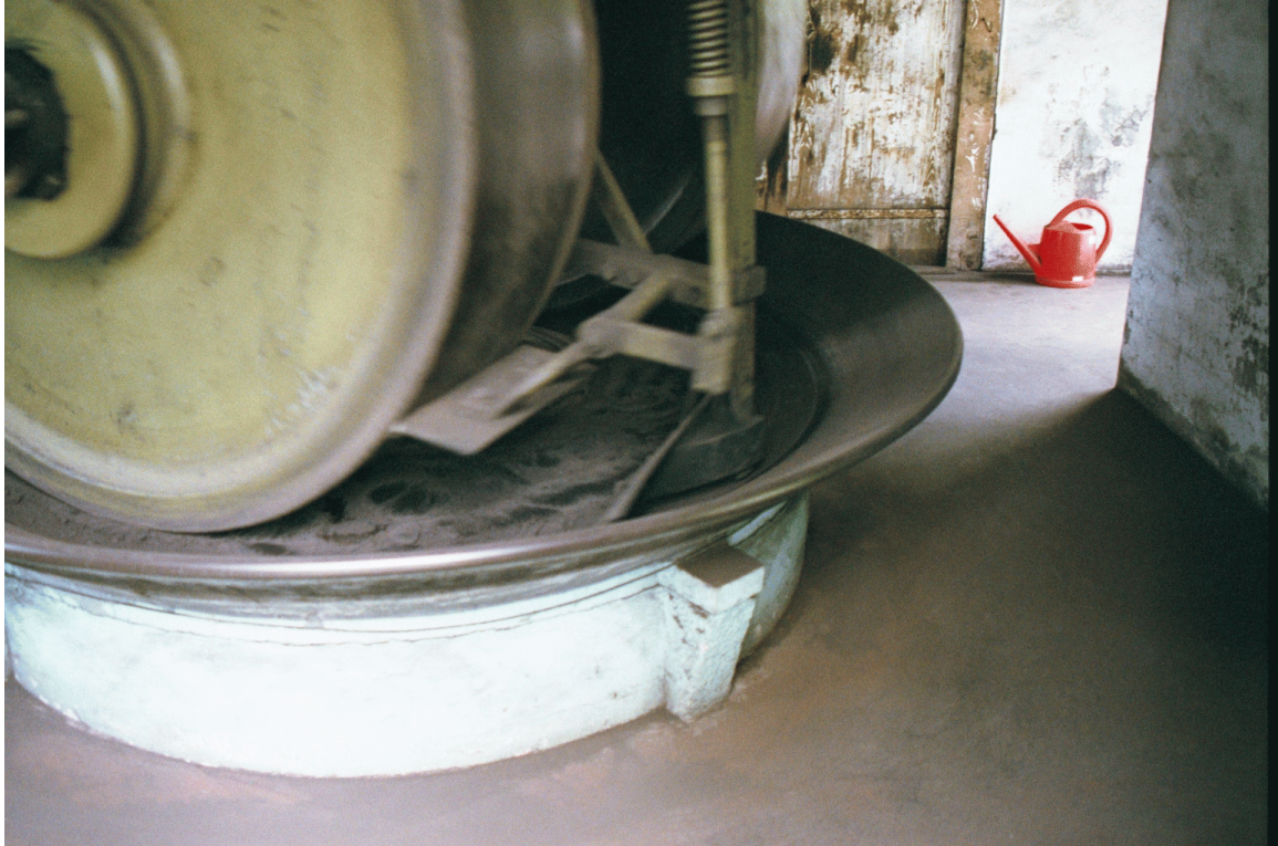
Figure 24. View of wheel scraper and batch plough.
