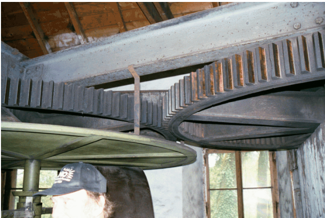
Figure 19. Overhead mill drive gears.
