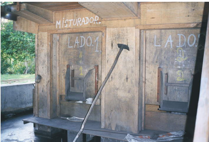
Figure 64. Outlet hatches for the finished powder.
