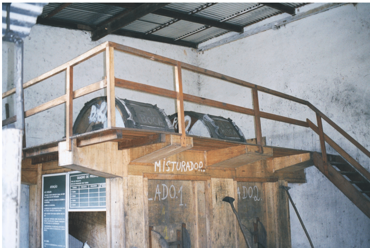
Figure 62. Polishing barrels in their stand.
