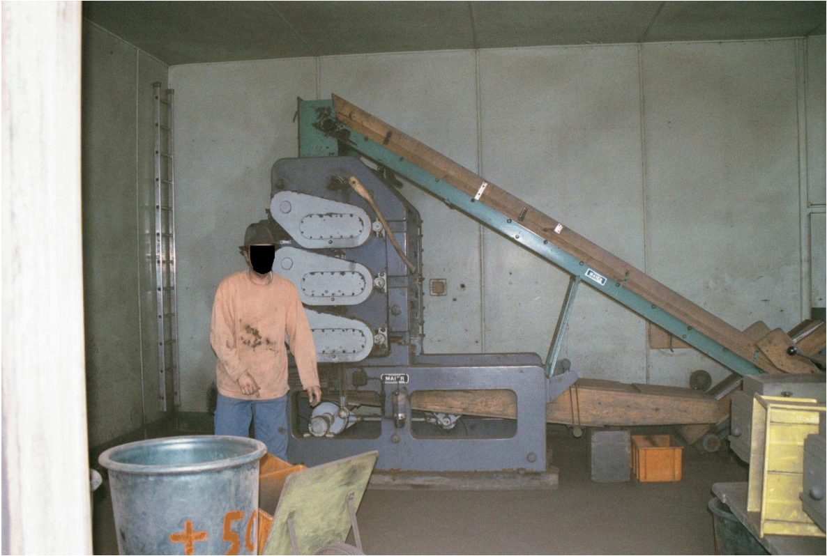
Figure 48. Corning mill in the Swiss black powder plant using 3 pairs of rolls.
