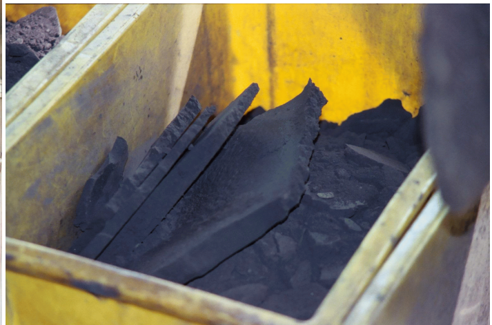
Figure 44. Pressed powder cake from the press.
