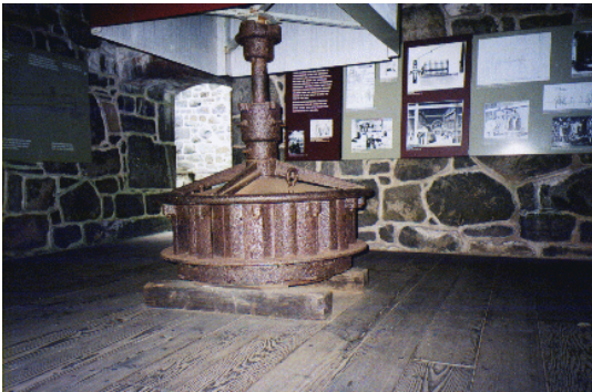
Figure 30. Water turbine rotor.
