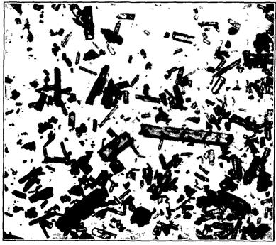
FIGURE 49. Commercial Sample of Ammonium Picrate (25×).
