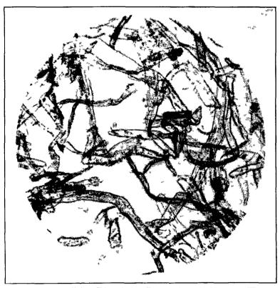
Figure 62 Nitrocellulose Fibers before Beating (132×) (Courtesy Western Cartridge Company)
