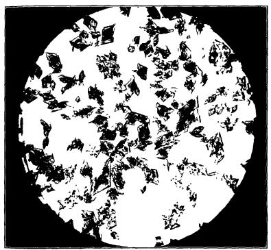
FIGURE 94. Mercury Fulminate Crystals for Use in Printer Composition (30×).
