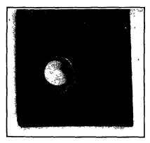
FIGURE 16. Effect of Detonator on Lead Plate 10 cm. Distant from Its End. The diameter of the hole is about 1½ times the diameter of the detonator which was fired. The lead has splashed up around the hole in much the same fashion as placid water splashes when a pebble is dropped into it. Note the numerous small splashes on the lead plate where it was struck by fragments of the detonator casing.
