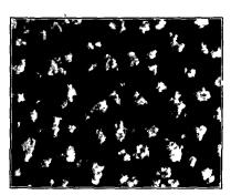
FIGURE 58. Nitromannite, in Grained Form for Charging Detonators (5×). (Courtesy Atlas Powder Company.)
