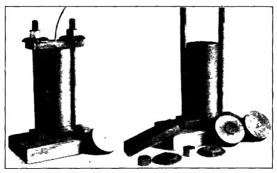
FIGURE 98. U. S. Bureau of Mines Sand Test Bomb No. 1. (Courtesy U. S. Bureau of Mines.) At left, assembled for making the test. At right, disassembled showing the parts. Two covers, one with a single hole for miner's fuse, the other with two holes for the two wires of an electric detonator.
