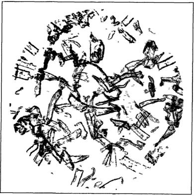
Figure 63 Nitrocellulose Fibers after Beating (132×) (Courtesy Western Cartridge Company)
