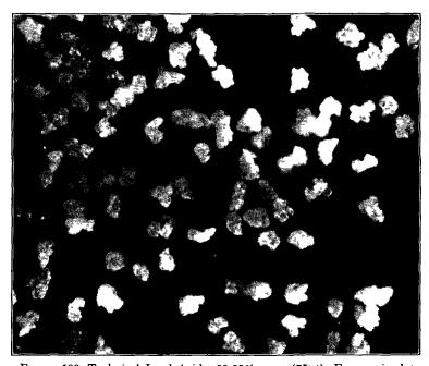
FIGURE 100. Technical Lead Azide, 90-95% pure (75×). For use in detonators. Precipitated in the presence of dextrin, it shows no crystal faces under the microscope.
