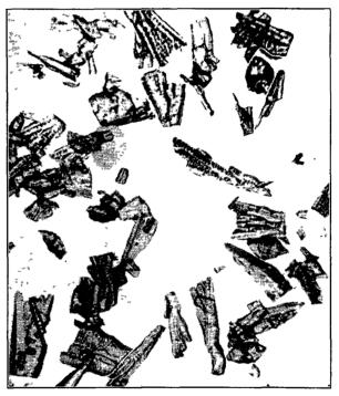
FIGURE 104. Tetracene Crystals (150×).
