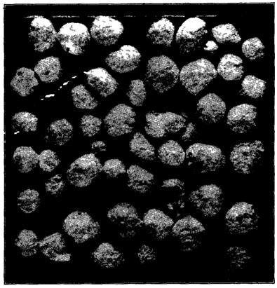
FIGURE 70. Shreddy Grains of Bulk Powder (25×). (Courtesy Western Cartridge Company)
