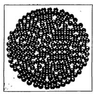
Figure 81. Ball Grains (Smokeless Powder) (3×). (Courtesy Western Cartridge Company.)
