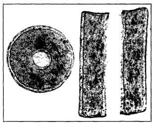
FIGURE 80. Cross Section and Longitudinal Section of a Grain of .50 Caliber Extruded Smokeless Powder, Deterrent Coated (25×). (Courtesy Western Cartridge Company.)
