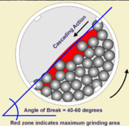
Figure 2: Optimal angle of break for cascading action.
