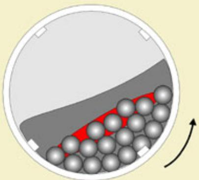
Figure 4: Undercharged media with overcharged load.
