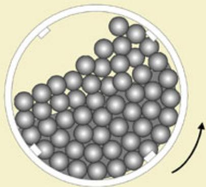
Figure 3: An overcharged mill.
