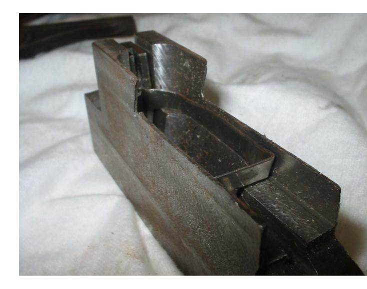
After the hammer/ sear slots are done you can use a file to square up the rear of the mag slot and get it fitting up through the block.
