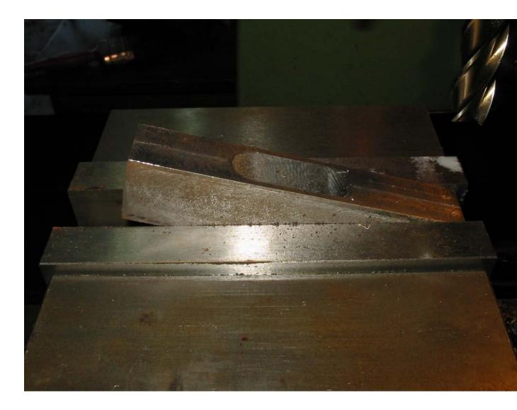
Getting your measurements from the blueprints remove the excess materials to leave you with the shape as per the sketch. I use a 9" grinder with cut off wheels to remove most of the materials and to get a lot of the slots hogged out undersized before final milling to save a bit of time.
