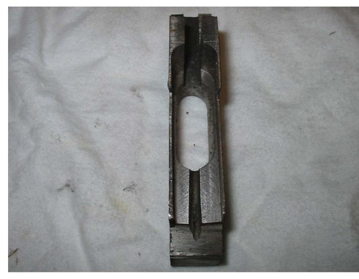
All going well your trigger should now fit in the slot you just cut and the "top" edge of the trigger bow is the correct distance from the top edge of your block where the rails will be. (IE, 0.64 below the link pin hole centre)
