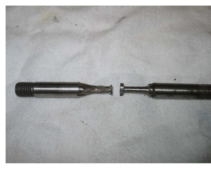
On the right is the slot cutter for the MS housing slots which is also useful in the safety catch undercutting.
