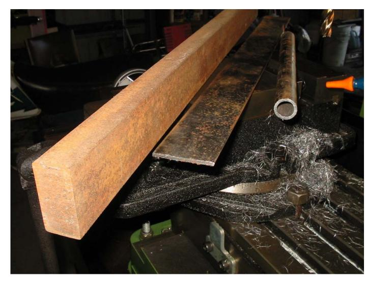
I start of by squaring up the top and the front of the rail block in the mill to provide surfaces to measure from.
