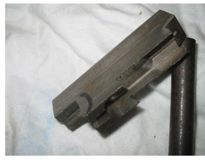
Back to the mill and now is the time to mill out the barrel link area and then cut the trigger bow slot in the bottom side of the upper rail block as well as the trigger slot itself.
