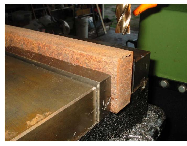
Then put some light layout lines for the barrel link pin position or measure it all from the front edge and then mill the start of the mag slot to give a flat surface at the required 17.5 degrees, drill the front of the mag slot and mill out the remaining material with a long series mill cutter.
